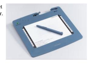
MeetingPad and software works with current versions of Windows and with Mac OS X software. There are two models: a Bluetooth and serial version. The Bluetooth version (Model 400) costs a bit more and provides the Bluetooth interface and rechargeable lithium-ion batteries, which allow approximately 40 hours of use between recharges. The Bluetooth-enabled version of the pad weighs less than two pounds and costs \$585.
